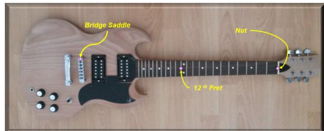
Distance from Bridge to 12 th fret = Distance from 12 th fret to nut
